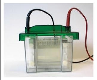
The image above shows a model BioRad Mini-PROTEAN II Electrophoresis Cell, the type of apparatus used for this experiment. The pre-cast BioRad Mini PROTEAN 10 well gels were used for resolving the proteins by size, shape and charge down the gel in order to determine protein size (in kDa). The cell was plugged into a power source and run in SDS buffer for 90 minutes at  $160, \pm 2.0 \text{ V}$  with constant amperage.
