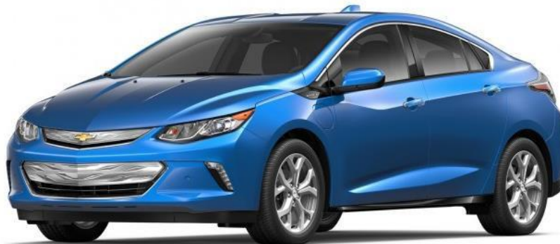
2016 Chevrolet VOLT - electric vehicle with gasoline powered range-extending capability (EREV).
